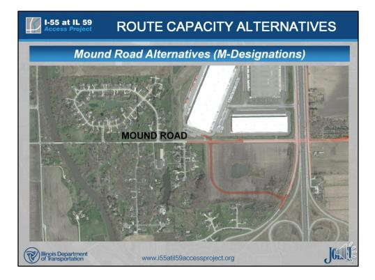
Three alternatives were developed to address Mound Road capacity and connectivity, referred to as M-Designations. All are being recommended for elimination from further study.
