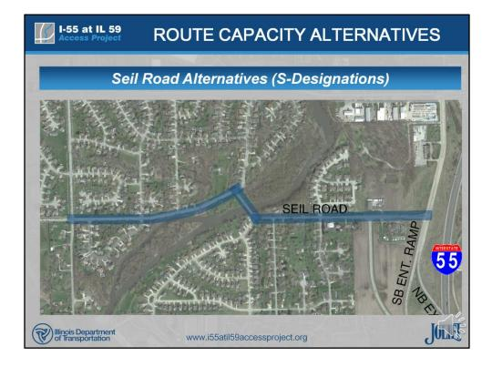
Six alternatives were developed to address Seil Road capacity, referred to as S-Designations. All are recommended for further study.
