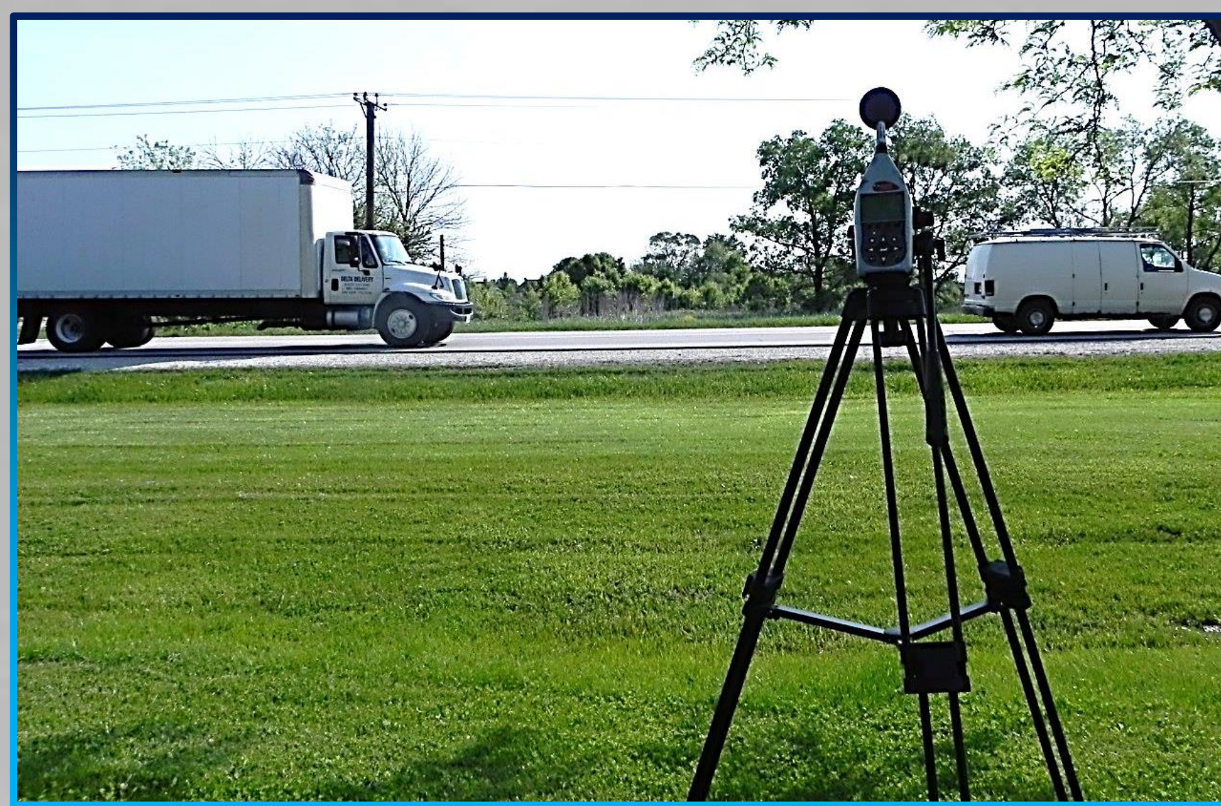
Traffic Noise Field Measurement
